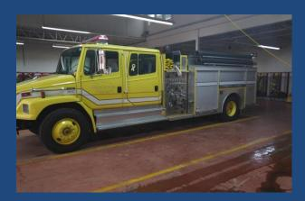
T1 (9734)-2007 E-One Navistar Hale 500 gpm fire pump 2000 gal. On board water tank
