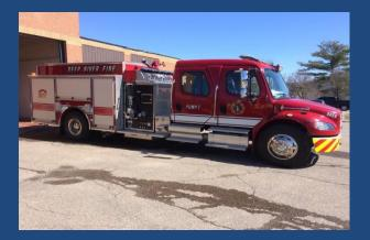
P1 (9668) – 2013 Pierce Freightliner Waterous 1250 gpm fire pump 850 gal. On board water tank Fire Profoam system
