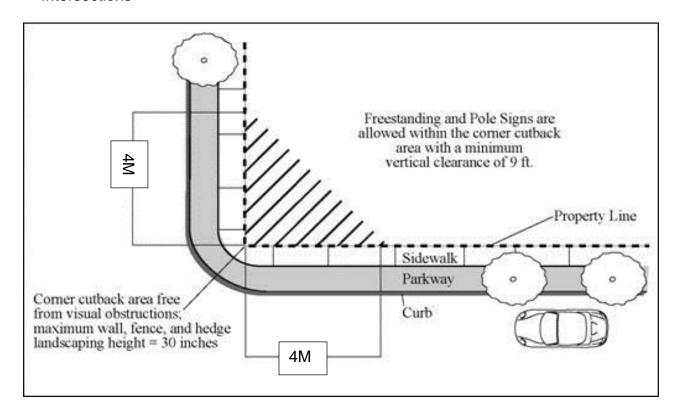
The above diagram highlights the area at an intersection that must remain free of any non-regulatory signage. The purpose of this is to ensure good visibility and safety at all intersections.
