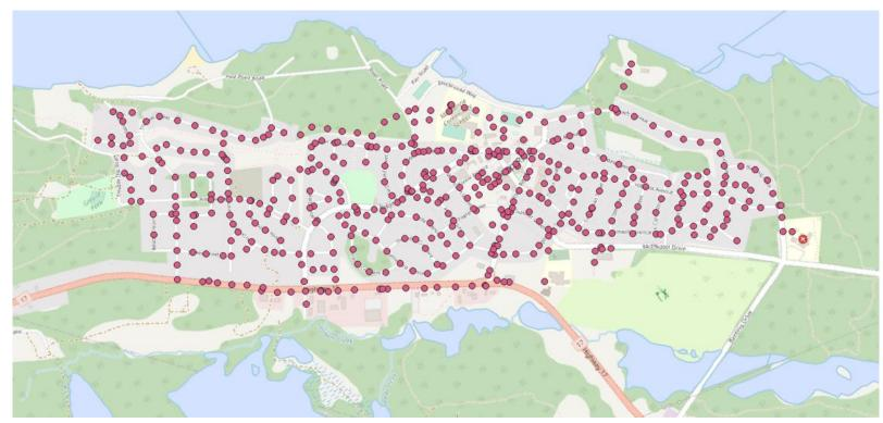
Figure A - 17: Sanitary Maintenance Hole Asset Map
