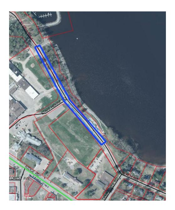
The scope of this project consists of rehabilitation through mill and pave of 350 meters of Brockhouse Way (Entrance of Cockcroft Residence to Entrance of Town water access/boat launch). In order to complete this section four culvert outlets will be replaced as well as widening the road from the current 6.2 meters to 7 meters. Lastly, the 8-vehicle parking lot to Riverbank Park, along Brockhouse Way, will be rehabilitated as part of the project.
