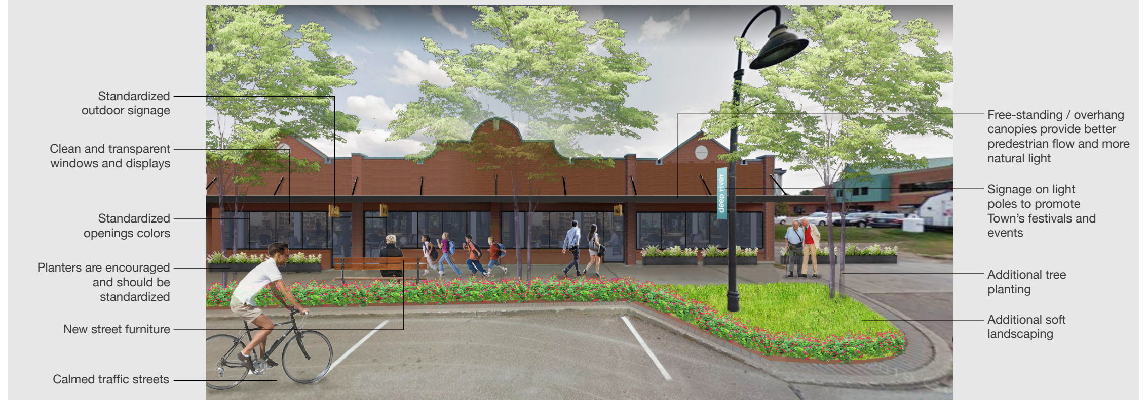
Figure 70c: Demonstration of Architecture Controls on retail facades along Champlain St. Source: Fotenn sketches over Google image.
