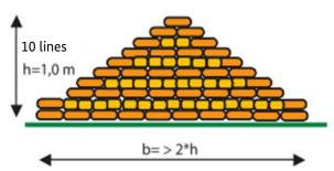
The sandbag dam should always be laid in a dense bond so that it is virtually impermeable. The use of film on the water side has also proved its worth.
